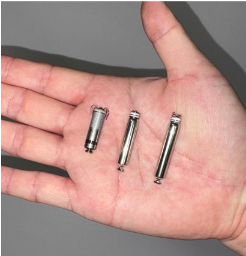
Figure 1. Currently available leadless pacemakers. From left: Micra™ (Medtronic), a tine-based leadless pacemaker; AVEIR AR™, and AVEIR VR™ (Abbott), screw-based leadless pacemakers.
